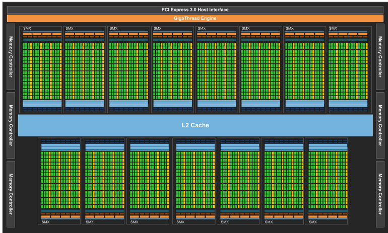
Nvidia Kepler architecture (full GK110)
