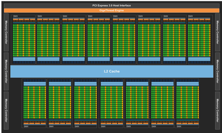
Nvidia Kepler architecture (full GK110)
